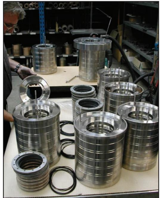
■ (Left) Complete rod packing cases with lubrication, cooling, vent and buffer gas connections. (Right) Rod packing case assembling.
