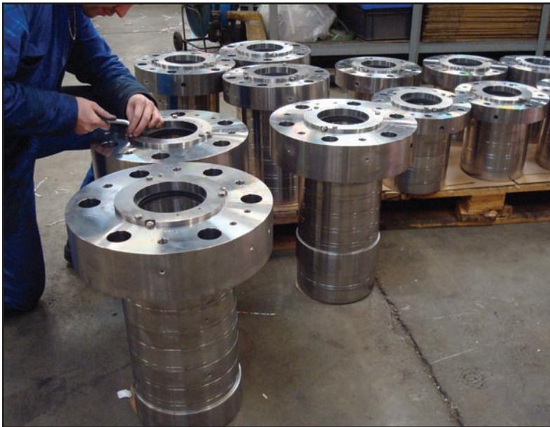
■ Complete packing cases for a rod diameter of 5.31 in. (135 mm), before shipment.
